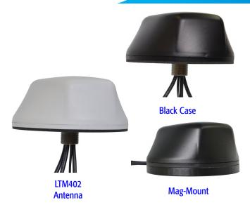
Mobile Mark's LTM402 Series antenna contains four separate antennas, all in one compact antenna housing: two Global LTE/Cellular antennas, one 2.4/5 GHz dual-band WiFi antenna, and one GPS antenna. The LTM402 differes from the LTM401 in that it covers all LTE systems worldwide from 694-3700 MHz.
