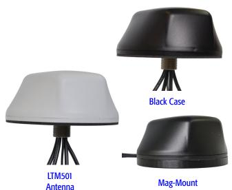
Mobile Mark's LTM501 Series Multiband Diversity/MIMO antenna contains five separate antennas, all in one compact antenna housing: two LTE 700 MHz & Cellular antennas, two dual-band WiFi antennas, and one GPS antenna.
