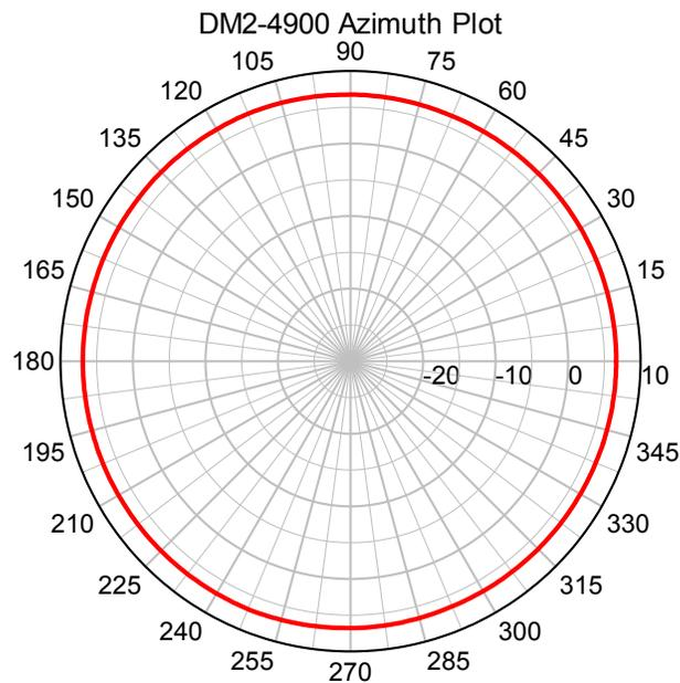
Note: Azimuth Plot is at an elevation angle of 156° for the coordinate system shown above.
