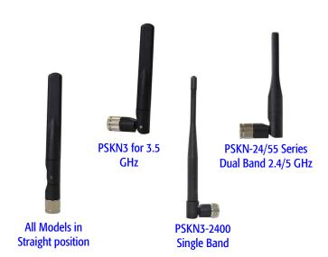
These 1/2 wave antennas require no ground plane for operation. This makes them ideal for use with portable devices or products with no substantial ground plane. They can even be used with products that consist of all plastic chassis or case.
