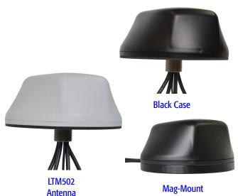
Mobile Mark's LTM502 Series Multiband Diversity/MIMO antenna contains five separate antennas, all in one compact antenna housing: two broadband LTE/Cellular antennas, two dual-band WiFi antennas, and one GPS antenna. The LTM502 differs from the LTM501 in that the broadband LTE/Cellular element covers all LTE frequencies worldwide, from 694-3700 MHz.
