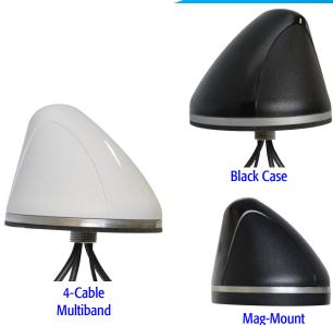
The SMW-412 Series Antennas features 4 elements in one antenna radome. The unique feature of this model is that the cellular element (Cable 1) is extremely widebanded and can cover: LTE at 700 MHz as well as the established 850/1900 GSM/CDMA bands, 1.7/2.1 AWS bands and WiMAX 2.5 all on a single board.
