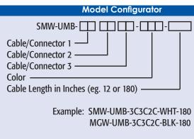
Specify "SMWG" or "MGWG" instead of "SMW" or "MGW" for GPS/Glonass combination antenna.
