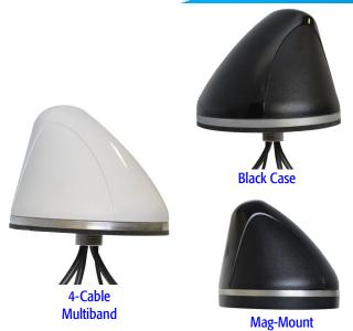
The SMW-414 Series antennas features 4 antenna elements in one radome. The unique feature of this model is that the cellular element (Cable 1) is extremely widebanded and can cover the traditional GSM/CDMA frequencies, 700 MHz LTE, 1.7 & 2.1 GHz AWS/UMTS and LTE/WiMAX at 2.5 or 3.7 GHz, all on a single board.
